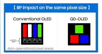
The switch for each pixel occupies a certain area. When the size of each sub-pixel is reduced for high resolution, the area blocking the light becomes relatively larger, results luminance loss. On the other hand, the 'Top emission' structure of QD-OLED does not have blocked area, so there is no effect of BP even if the pixel size is reduced.
